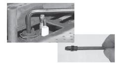
Remove burner orifice with a 1/2" wrench. Use another wrench to hold on to the elbow behind the orifice. Discard orifice.
